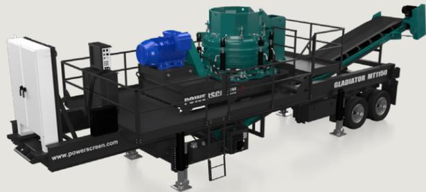
The Gladiator MT1150 is a new electrically driven, wheeled open circuit cone crusher. It features the renowned Terex (r) TC1150 cone chamber and is chassis mounted on wheels meaning ease of movement and quick set up times.
