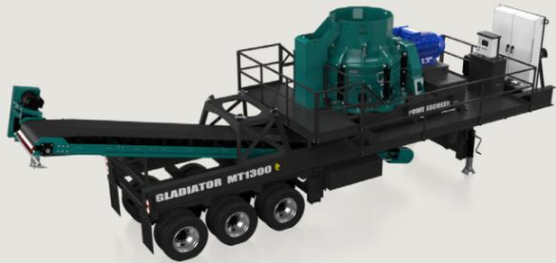
The new Gladiator MT1300 is an electrically driven, wheeled open circuit cone crusher. It features the tried and tested Terex TC1300 cone chamber and is mounted on wheels which ensures ease of movement and quick set up times.
