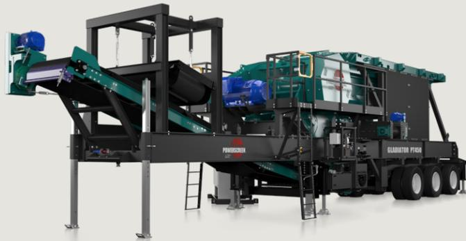
The Gladiator PT450 is a new electrically driven, portable jaw crusher. It features the tried-and-tested Terex CR040 jaw crushing chamber and is chassis mounted on wheels meaning ease of movement and set-up.
