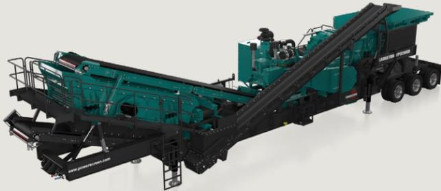
The Gladiator TP320SR is a new hybrid-electric drive, wheeled, closed-circuit impact crusher.
